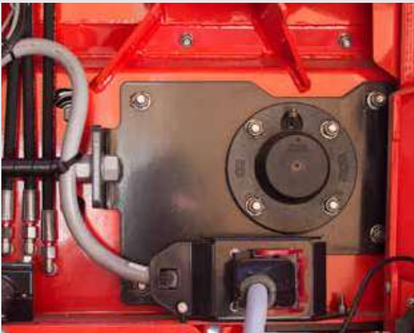
Sealed belt shaft bearing and quick coupling for the spreader unit electronics
