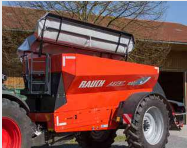
The hopper cover reliably protects the spreading material and can be effortlessly opened
