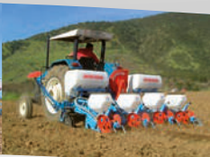
Multi-purpose pneumatic planter with NC shoes
